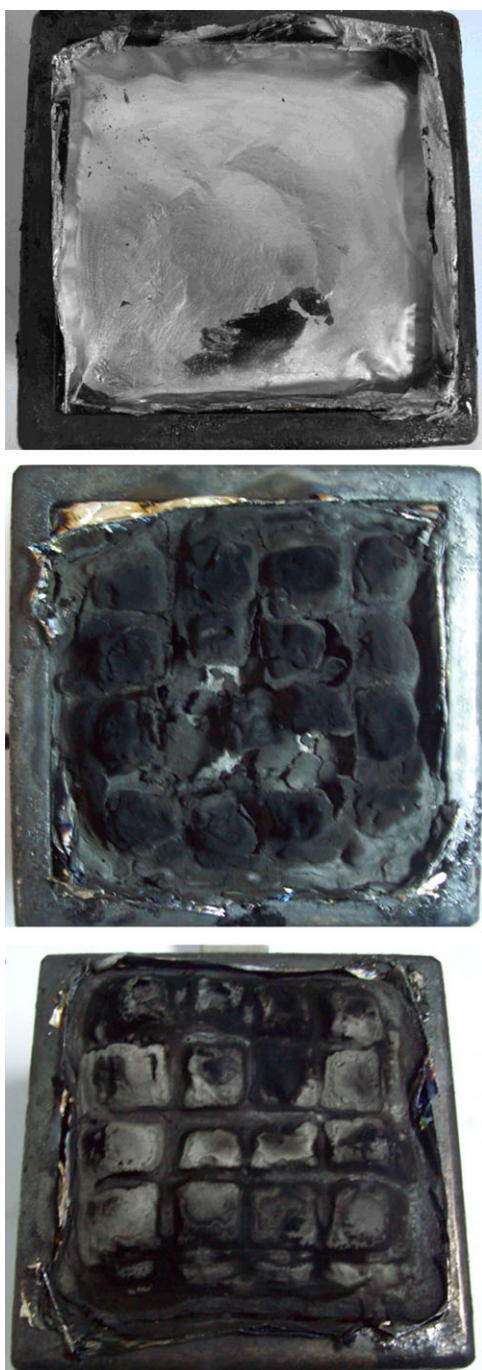
Figure 5. Morphologies of the residues produced from the composites after cone calorimeter test. [Color figure can be viewed in the online issue, which is available at wileyonlinelibrary.com ]
